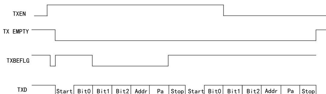
Figure 204 Transmitter Signal Timing
